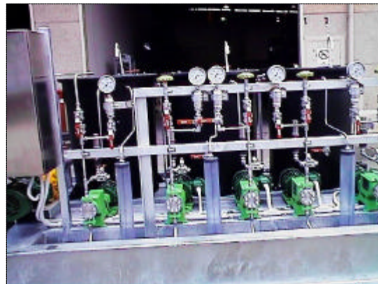
Similar to the units bound for Goro Nickel is the Kelair-designed metering package (pictured above and below) built for Perth's Worsley Alumina.
